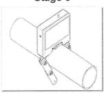
The unit should be located on the cold water pipe to where the water is being heated in the boiler. (see over page)
